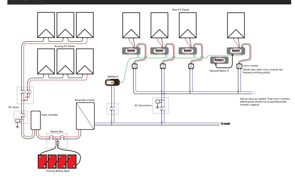
As long as your existing inverter has a reversible ability (most of quality inverters do), you can connect Panel + Batsol + Micro-inverter units on the AC side. This allows to increase PV power, storage and AC power altogether. Support : info@batsolpower.com
