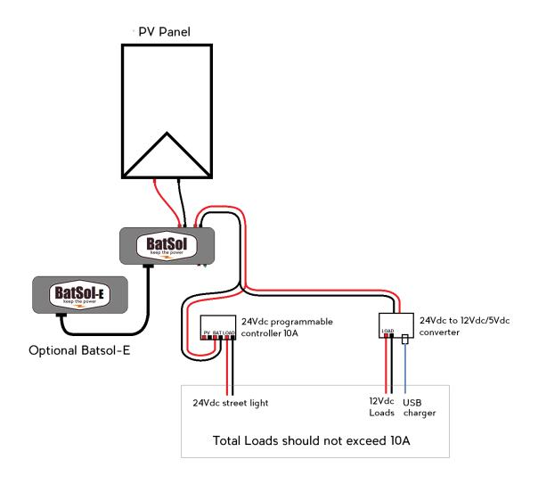
Batsol can easily be used to power up lighting units or DC loads up to 240W. As Batsol has an intergrated BMS, it will not over or undercharge. The 24Vdc programmable controller is only used to set lighting hours or other load driving features. Ouput voltage range of the Batsol is 24Vdc to 32Vdc. Make sure your device can meet these values. Support : info@batsolpower.com
